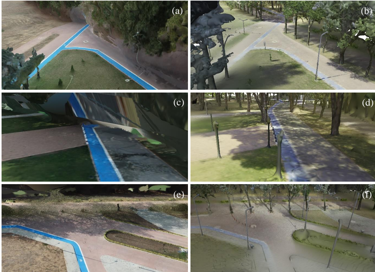
Figure 3: Digital twins generated from the UAV point cloud (a) (b) (c) and digital twins generated from the fusion of the UAV and TLS point clouds (b) (d) (f)
