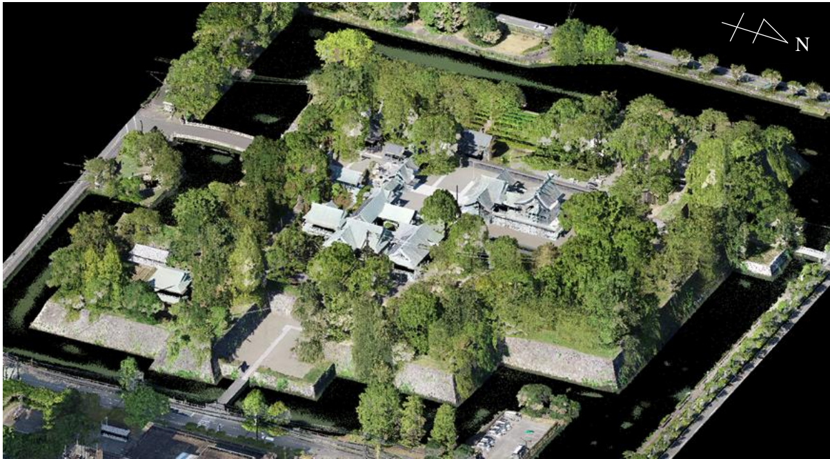
Figure 1: Aerial view of Hon-maru (main enclosure) in Yatsushiro Castle Ruins (UAV LiDAR point cloud)
