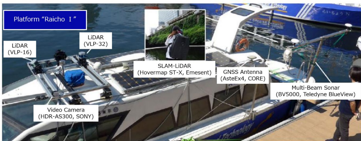
Figure 5: Experimental equipment for point cloud acquisition.
