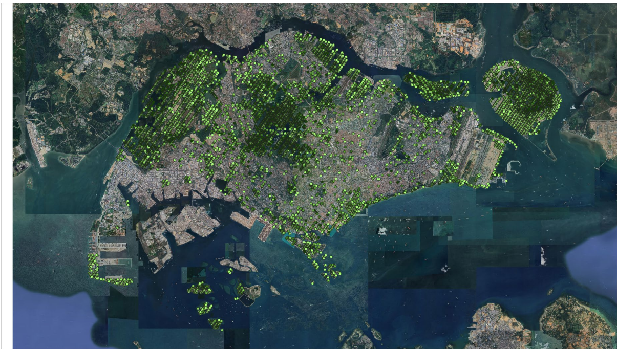
Figure 2: GEDI footprints and the corresponding data coverage for estimating AGBD and canopy height within the study area with darker greens showing higher AGBD. Footprints are not to scale.
