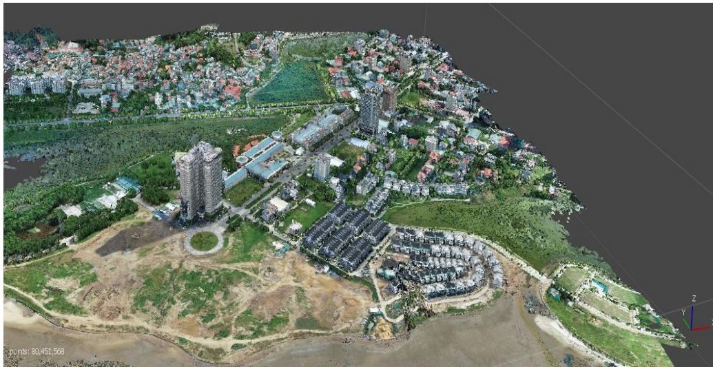
Figure 1. Point cloud constructed from UAV images in the experimental area
