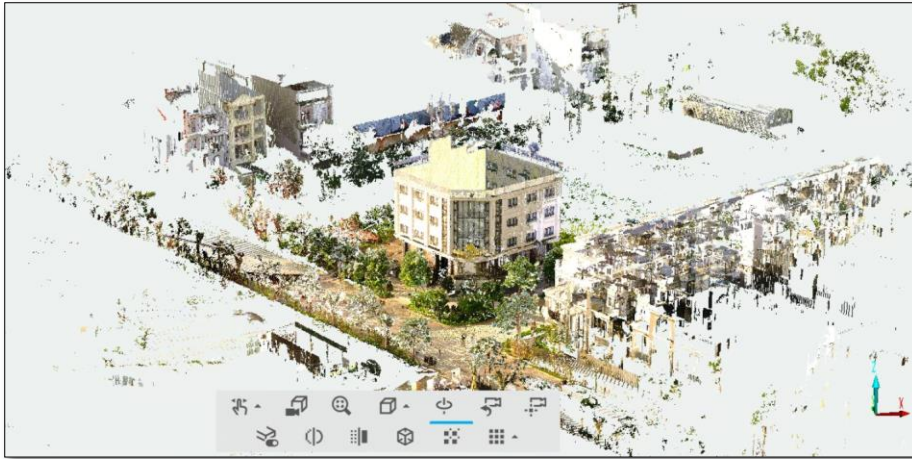
Figure 6. TLS point cloud for a detached house
