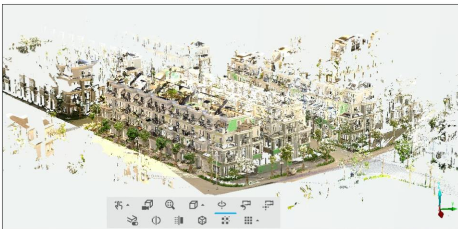
Figure 7. TLS point cloud for row of adjacent villas
