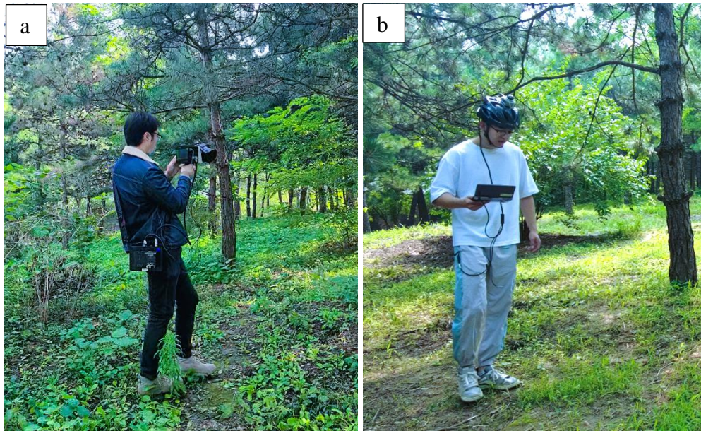
Figure 2: Photographs of (a) the handheld MLS (GoSLAM RS100) and (b) the helmet-mounted MLS (AIRCAS HM1) in coniferous plot.
